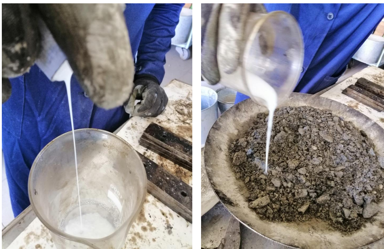
Figure 3.2 – Preparing the mixture, adding additive Nanoalps System SOIL
