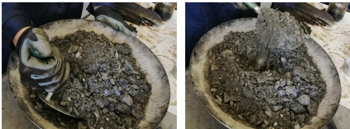
Figure 3.1 – Preparing the mixture
