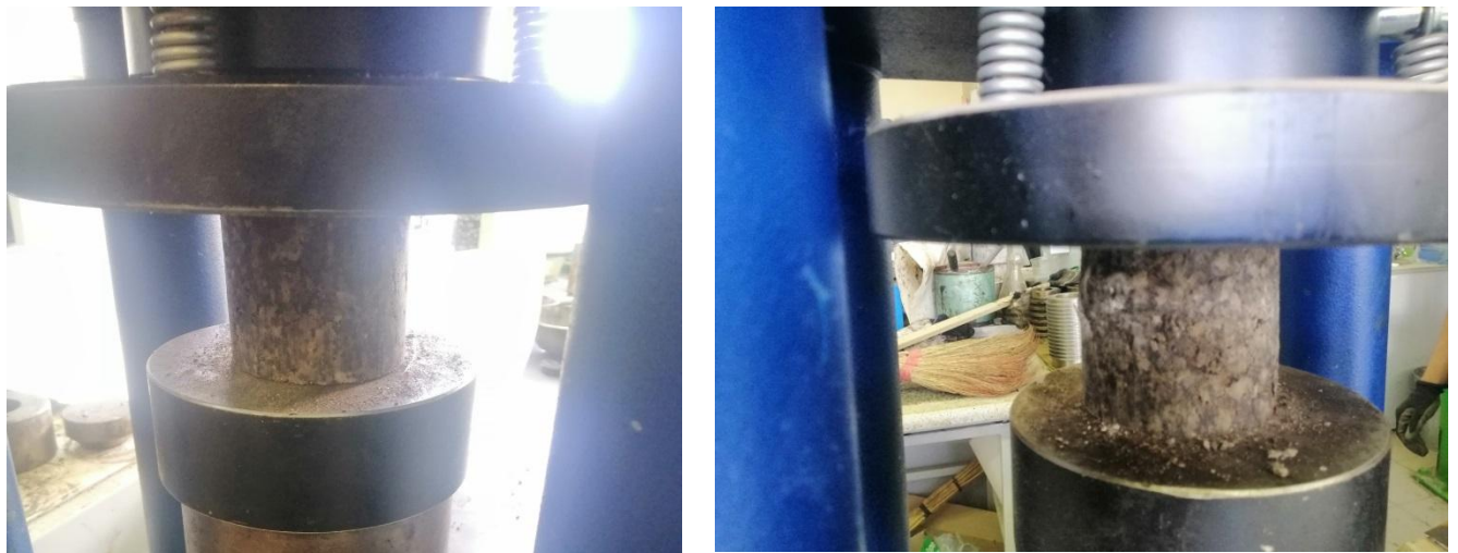
Figure 3.5 – Determination of the compressive strength
